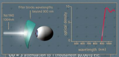
This filter is only effective at wavelengths above 900 nanometers. Such protective eyewear has a very high optical density for radiation of Nd:YAG lasers (1064 nm) but does not protect the eye against visible (400 - 700 nm) wavelengths!
