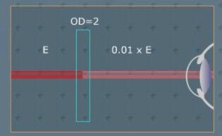
Laser protective eyewear reduces the ocular exposure at certain wavelengths.
