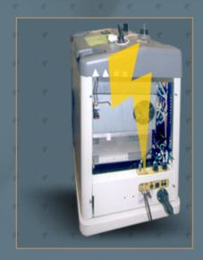
The efficiency of a laser system describes the conversion of electrical energy into optical radiation. If a laser output power of 1 Watt is required, the laser system needs [considerably] more electrical power. Laser diodes have the highest efficiency of all laser types at up to 40 %, a CO2 laser can reach 15 %, a Nd:YAG laser a maximum of 10 %. Other lasers transform less than 1 % of electrical power into light.
