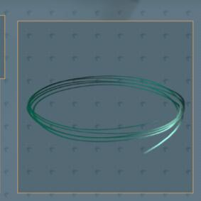
Hollow fibers are glass fibers with a hollow core. In contrast to solid fibers, they are capable of transporting infrared radiation which would normally be absorbed in glass fibers. Beams emitted from hollow fibers are highly divergent.
