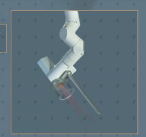
In order to deli be directed by Fibers made of various types of glass are only practical for wavelengths from about 350 to 2100 nm. Beams emitted from fibers are highly divergent.
