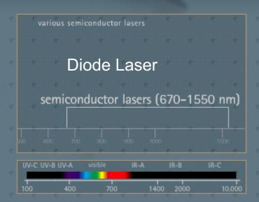
An [active medium] represents the 'heart' of a laser system. Gases, crystals, liquids and semiconductors are typical examples for such media.
