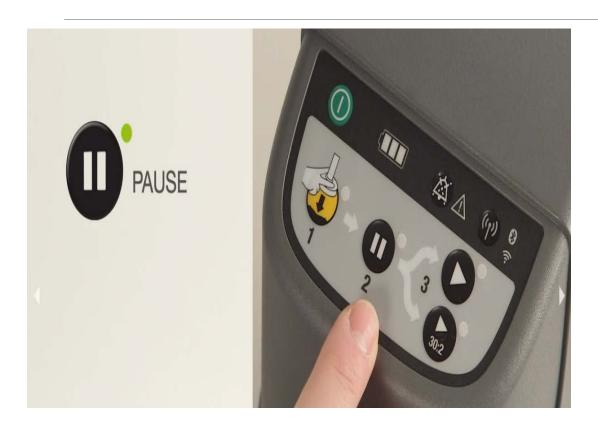
Press this button to lock the Piston in the start position.
