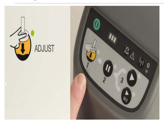
Once the unit is turned on, it automatically enters the adjust mode.
