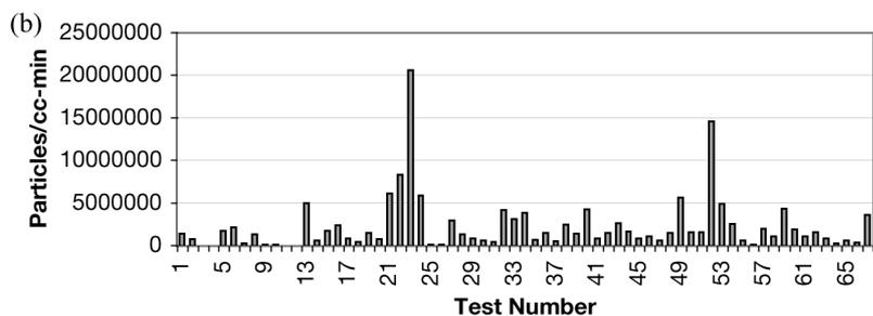
**Fig. 6.** (a) Average ultrafine particle concentration in 67 tests (>128 h). (b) Cumulative ultrafine particle exposures in 67 tests.
