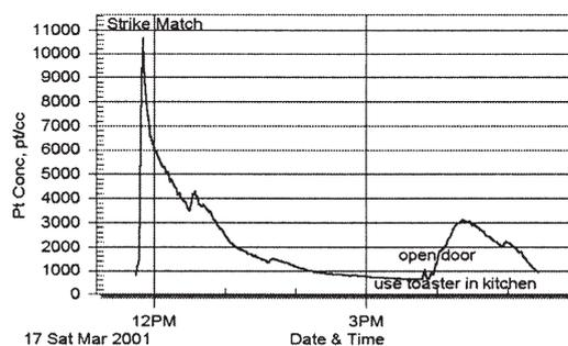
**Fig. 3.** Point source UFPM, decay and toaster UFPM dispersion.
