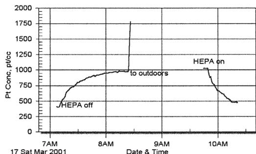
**Fig. 1.** Effect of a HEPA filtration unit in a residential home bedroom.
