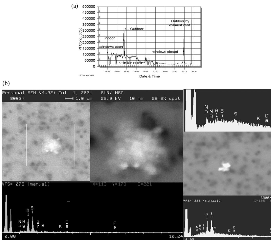
Fig. 4. (a) Re-entrainment of UFPM from kiln exhaust. (b) Examples of particles in kiln exhaust; 30 min sample. Aluminum silicate aggregate, sulfates (ambient) and zirconium silicate.
