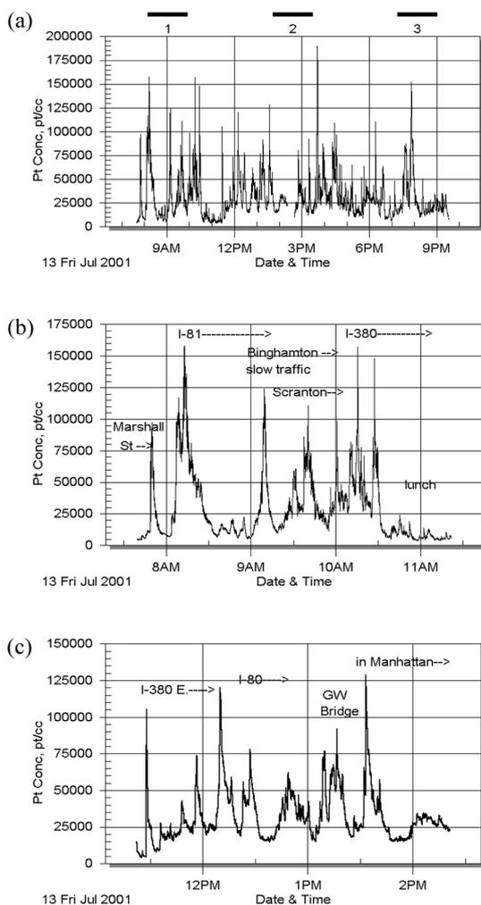
**Fig. 7.** (a) Long distance UFP exposure inside car: 13 h round trip, Syracuse to New York and back. (b) Syracuse to New York: UFP exposure inside car. Note the prolonged very high UFP levels related to variable traffic conditions in the city and on the highway. Longer time averaging does not reveal these. (c) UFP inside car in the vicinity of New York.
