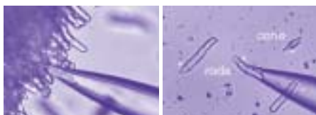
Electrode approaches rod photoreceptors protruding from the retina (left). By introducing part of a rod into the electrode, Dr. Solessio can record its response to light (right).
