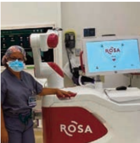
The robotic surgical assistant (ROSA) is used for minimally invasive brain surgery.
